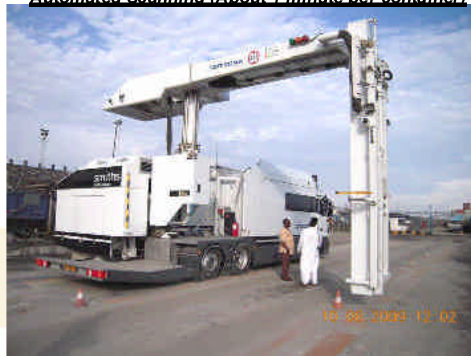
Automated Scanning (About 1 minute per container)
