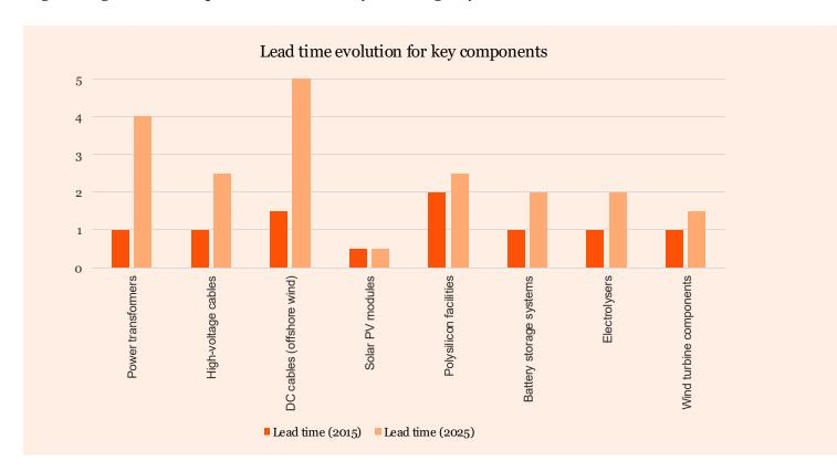
Source: IEA: Average observed lead time for permitting, construction and grid connection for selected energy projects.
