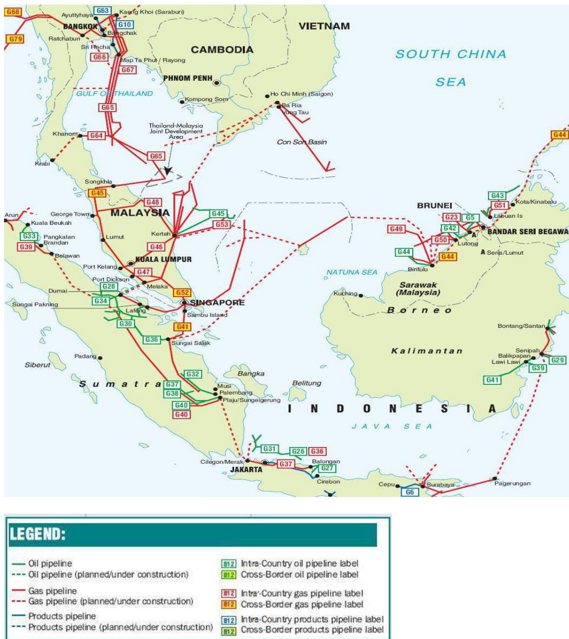
Figure L - 3: Map of Malaysia's Pipeline Infrastructure
