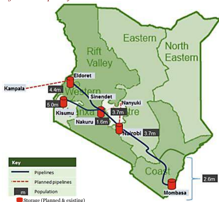
Figure 6.16: Pipeline fed terminals
