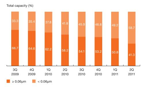
Fig. 10 Global semiconductor production capacity by feature size
