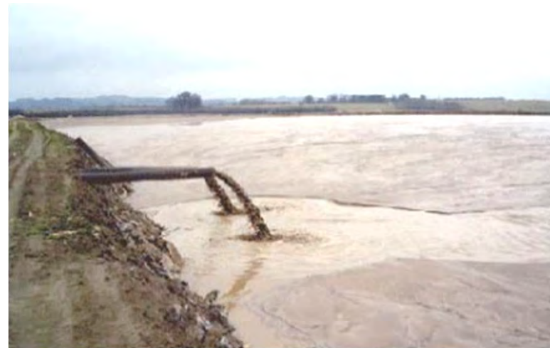
Single point discharge at Glebe Mines UK www.tailings.info/deposition.htm
