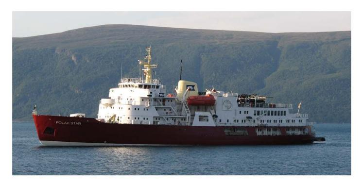
Originally named the Njord, the Polar Star was built as an icebreaker and meticulously operated and maintained by the Swedish Maritime Authority. In 2001, she underwent a complete conversion into an Arctic and Antarctic expedition cruise ship. The vessel is classed with DNV as a SOLAS compliant passengership with an Ice Class of 1A\*. The Polar Star is large enough to voyage to remote areas in comfort and small enough to enter out of the way destinations.
